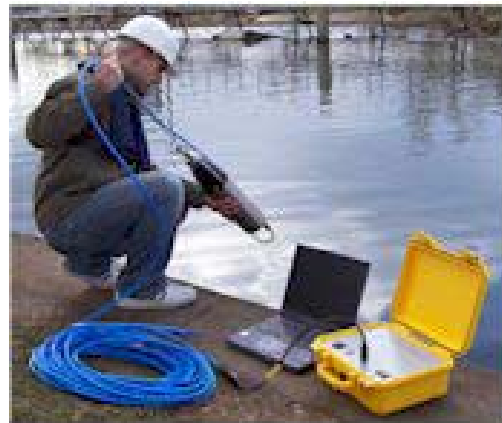
Fast tracka II sensor being deployed in a reservoir
